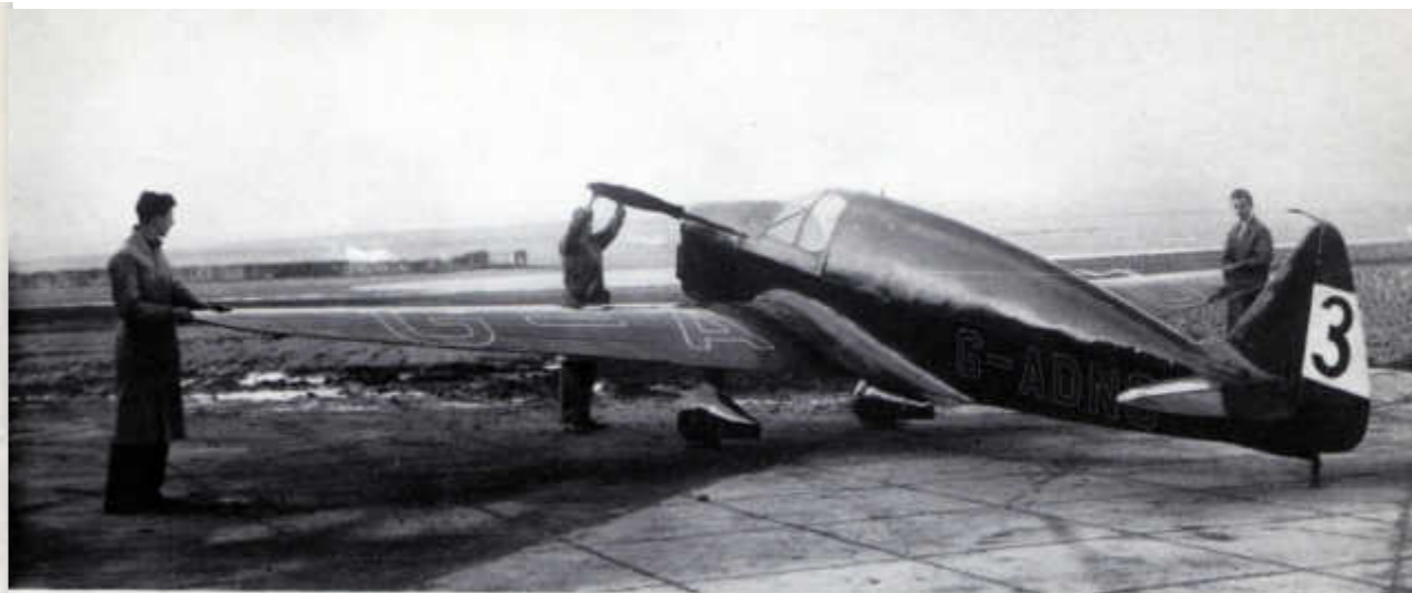
T.K.2. A high-performance single-seater designed and built entirely by de Havilland students. This aeroplane was placed fourth in 1935 and sixth in 1936 in the King's Cup Air Race. It also won the Heston to Cardiff Air Race in 1936 at an average speed of 189.2 m.p.h.
