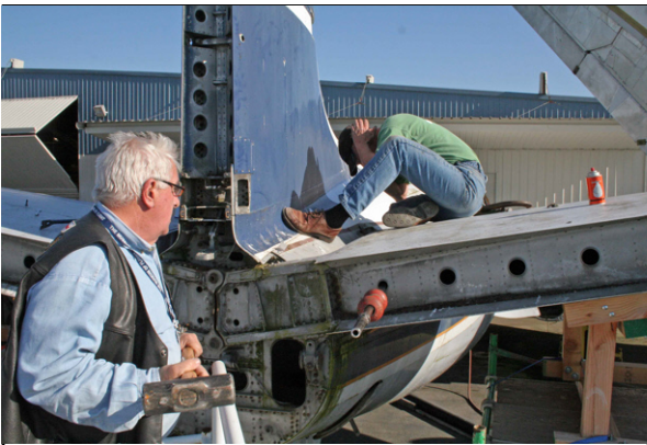
Jim Goodall with sledge hammer 'persuading' a pin to break loose while John Blum covers his ears.
