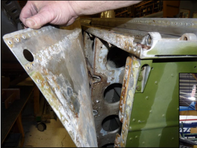
Horizontal stabiliser before restoration.
