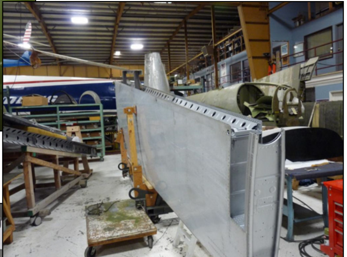
Horizontal stabiliser after restoration.
