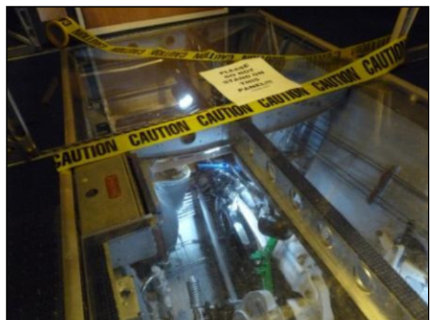
Figure 10 Aileron Control Bay viewed through its clear acrylic floor panel.
