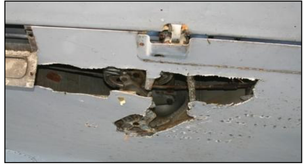
Figure 1 Corrosion Damage to wing bottom skin
