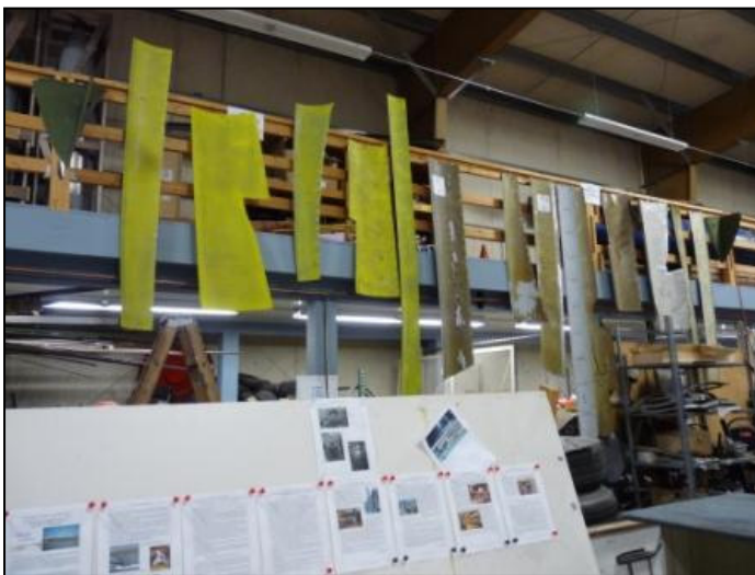
Figure 6 Wing root fairings under restoration.
