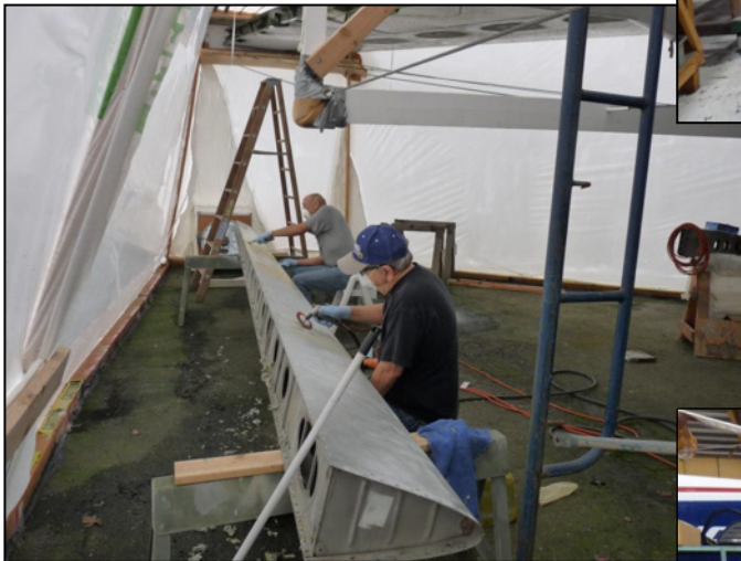
Part of vertical stabiliser under restoration.
