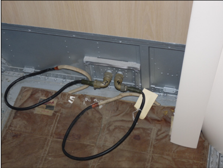
Center section under carpet floor heating "electric blanket" (important passenger comfort item, as the floor here is a pressure bulkhead and the fuel tanks below would track the -75 degree F OAT at altitude).
