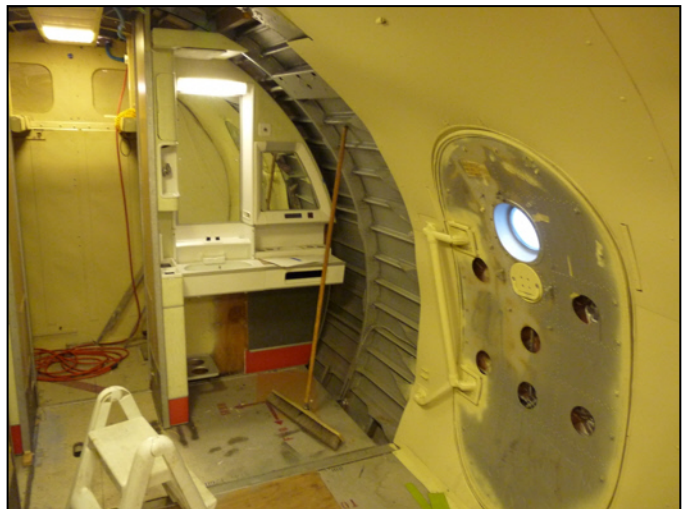
Advances in the port aft toilet and passenger door surround finish.
