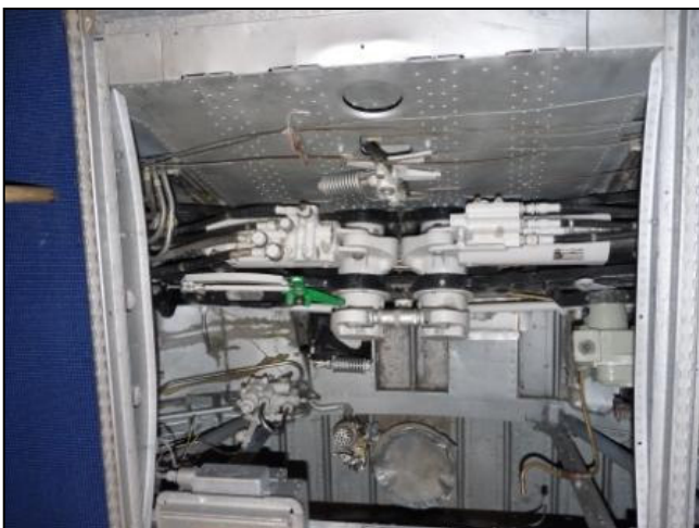
Figure 9 Aileron Control Bay under restoration.
