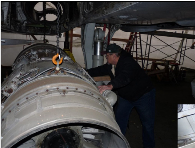
Above and left : lowering an engine.
