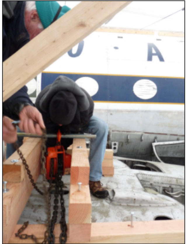
Above and left : lowering an engine.
