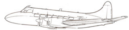
D.H. 114 Heron First flight 1950. 173 were built. Enlarged four engine development of the D.H. 104 Dove.
