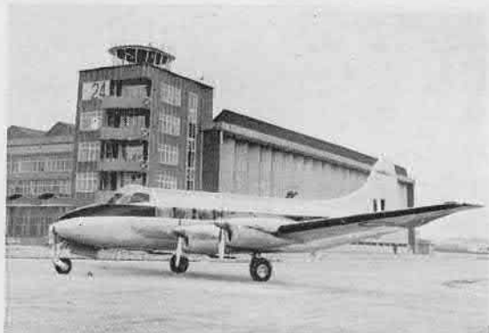
1950. The Heron feederliner with four Gipsy Queen 30 engines and de Havilland propellers.
