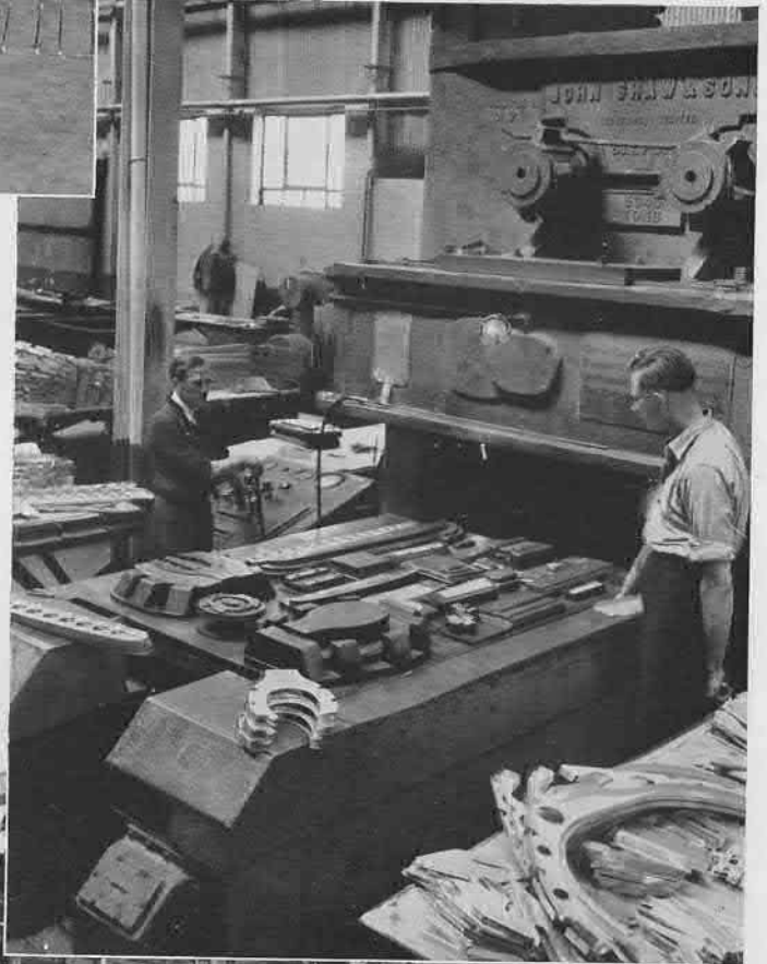
The rubber press is used to form many of the smaller sheet-metal components for aircraft.
