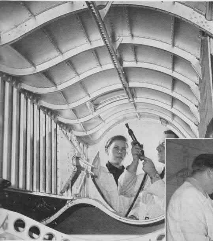
In the factories apprentices work with skilled operators who pass on to them the practical experience gained over many years. Here instructor and pupil are at work on the engine bay of a jet aircraft.
