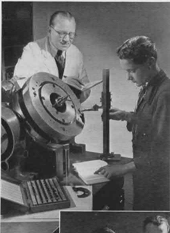
Metrology. Using a vernier height gauge and dial test indicator in conjunction with a dividing head.
