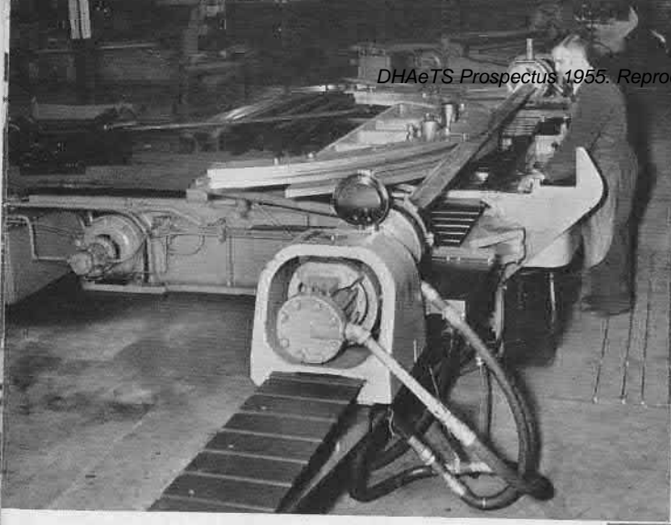
One of the battery of stretcher presses in the metal-forming shop.
