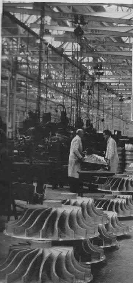
(Above) The production of jet engines, rocket engines and piston engines is centred at Leavesden. The department concerned with the machining of Ghost and Goblin compressors is seen here.
