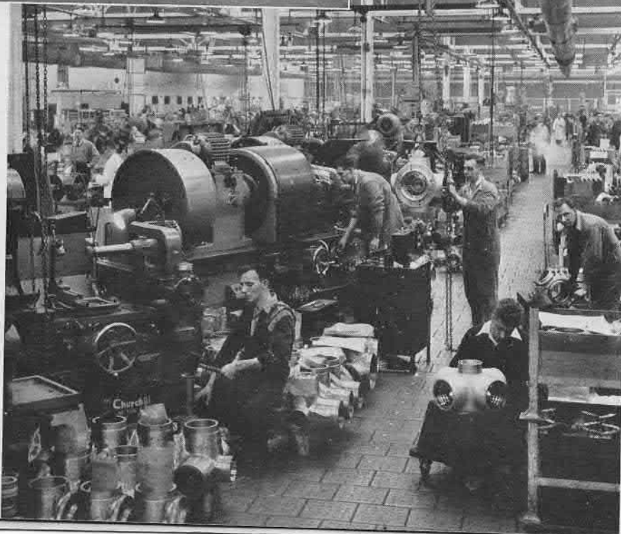
(Above) The production of jet engines, rocket engines and piston engines is centred at Leavesden. The department concerned with the machining of Ghost and Goblin compressors is seen here.
