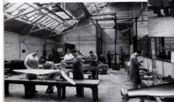
In the upper picture, students are shown checking balance and pitch of wooden air screws and finding the moisture content of timbers.
