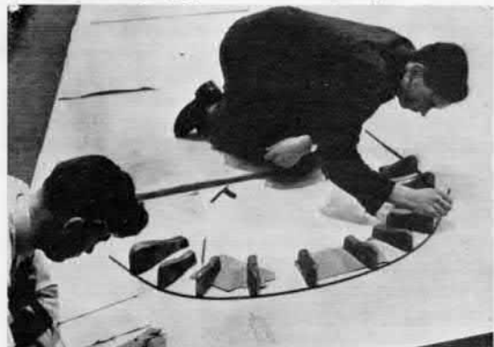
The lofting process in aircraft layout.
