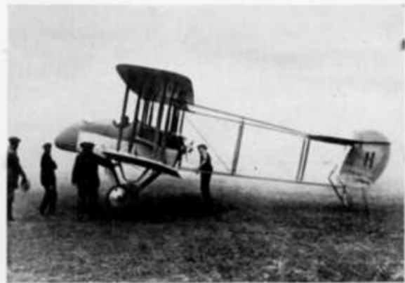
1914. The D.H.1 two-seat fighter designed at Hendon.
