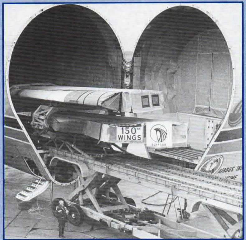
A set of Airbus wings being loaded onto a Super Guppy at Manchester Airport, for delivery to Toulouse.
