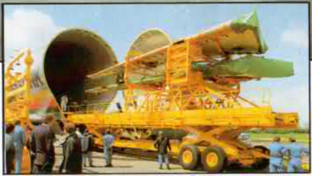
Airbus wings being loaded into a Supper Guppy for transportation to the final Assembly Line in Toulouse, France.
