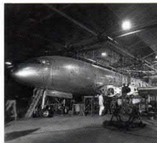
The Comet prototype under construction in the late 1940's.
