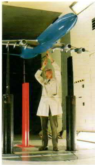
A scale model of the A340 in Hatfield's 15ft wind tunnel.
