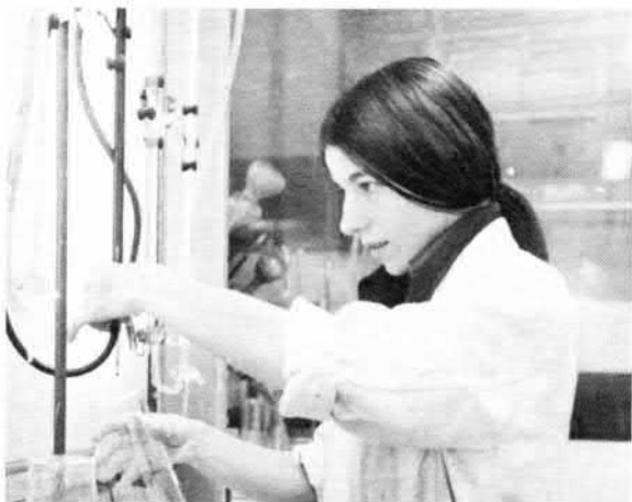
One of our laboratory technicians determining nickel content in a sample taken from the process plating plant
