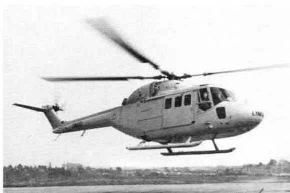
Two GEM engines power the Anglo-French Lynx helicopter
