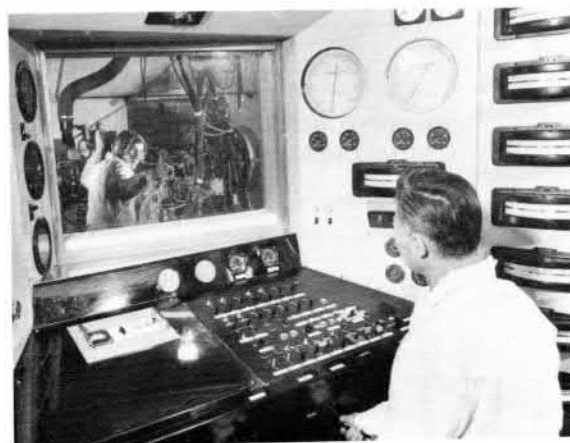
A gas turbine engine being subjected to a thorough test before delivery to a customer
