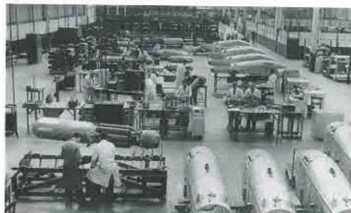
A general view of Super Sprite assembly work at the de Havilland Engine Company's production division where both the rocket and its nacelle are made. Each engine is given an endurance run on the test-bed before final assembly.
