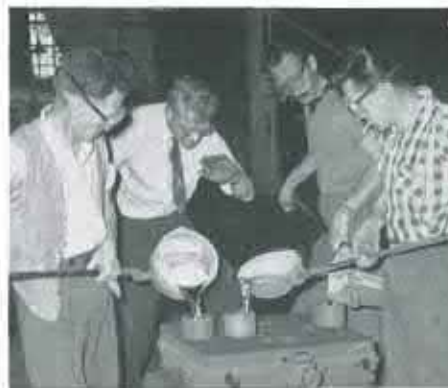
The Gnome intake casing is a casting in magnesium alloy by Kent Alloys Ltd., and it is shown here (below) being poured.
