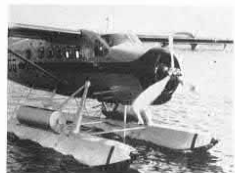
An Otter fitted with the new tanks and refilling device.
