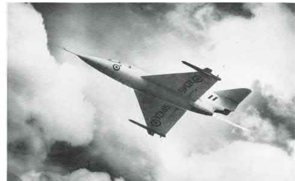
The Saunders-Roe S-R.53 aircraft fitted with Firestreak guided weapons, climbing rapidly on the power of its Spectre controllable rocket engine. The S-R.53 is actively engaged in a flight development programme directed towards the larger, operational S-R.177.
