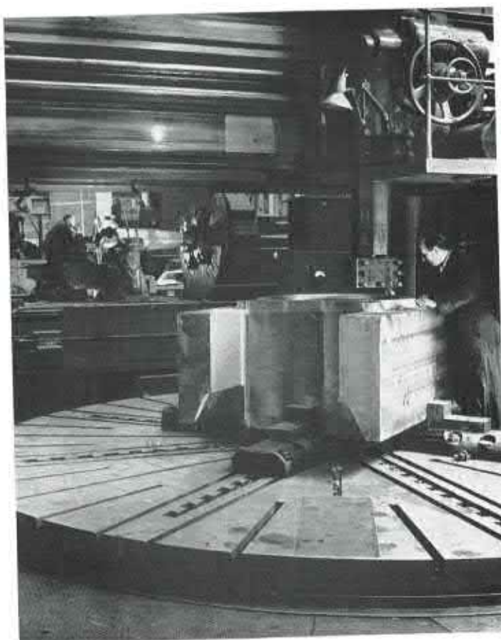
An intensive programme of work was laid down to accelerate the manufacture of the prototype engine, and in this respect it is interesting to note that it had already completed an unofficial acceptance run before drawings could be issued to the shops. Practical craftsmen with practised eye and a flair for improvisation were responsible for this — often, as is shown here, machining from the solid. In the foreground a rear bearing housing and, at the background, an accessory-drive quill shaft take shape from billets of high-tensile steel.
