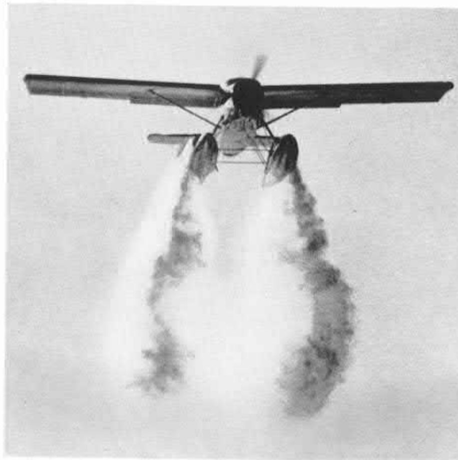
At the turn of a switch the tanks are revolved and discharge their load over the fire.
