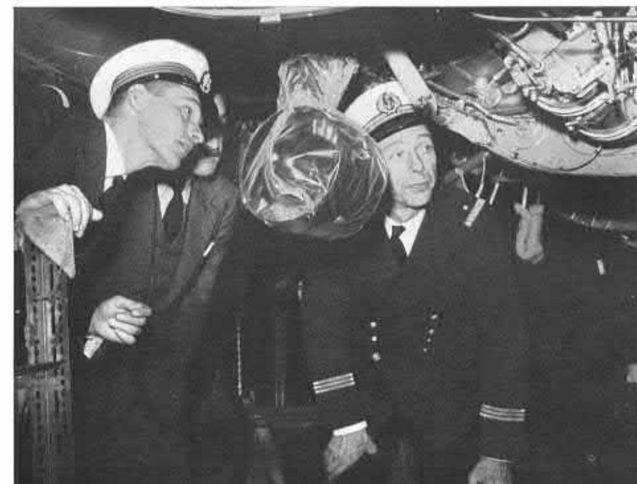
Headed by Capitaine de Corvette Mauban, a French Naval team has been evaluating the flying characteristics of the Sea Vixen. This photograph, taken at de Havilland, Christchurch, England, shows Lt. Landré (left) and Lt. Gérard (right) investigating the hydraulic system. In its plastic dust cap is the Plessey ram-air turbine which can be lowered into the air stream for the emergency operation of the hydraulic system.
