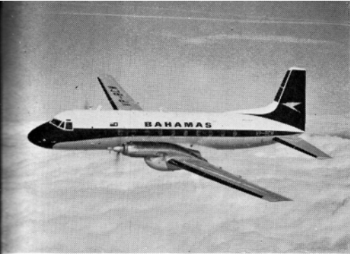
The HS 748, powered by Rolls-Royce Dart engines, seats up to 62 passengers and is in airline service throughout the world.
