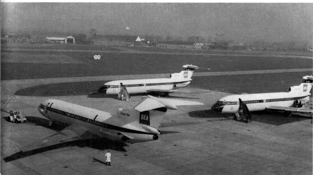
The longer-range Trident Two, now in production at Hatfield for British European Airways, is equipped for fully automatic landing in near-zero visibility.
