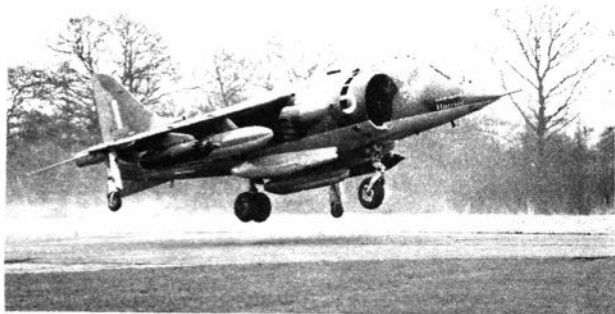
HS HARRIER The world's first operational V/STOL tactical strike fighter will enter service with the R. A. F. in 1969 - span 25 ft. 3 in.
