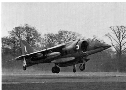
The Hawker Siddeley Harrier GR Mk I will be the first operational fixed-wing V/STOL aircraft in the world.
