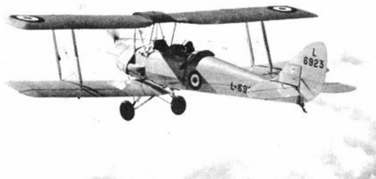
TIGER MOTH (DH82) An efficient primary intermediate and advanced training biplane - many pilots learnt to fly in the aeroplane - span 29 ft. 4 ins.
