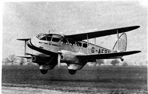
RAPIDE (DH89) The de Havilland twin engine express airliner - world famous - many built - span 48 ft. 0 in.
