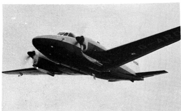
DOVE (DH104) Twin engine airliner in miniature - some 540 built - span 57 ft. 0 in.
