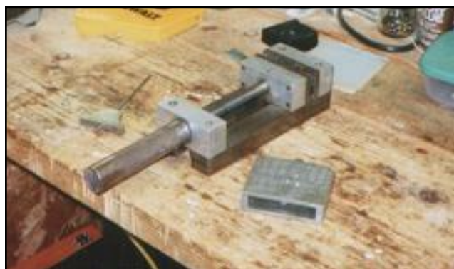
Some of Ray Yeoman's pristine tools, after 55 years of use. L to R, depth gauge, drilling vice, washer vice.
