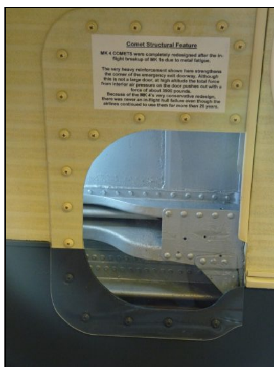
Reinforcement at corner of emergency exit.
