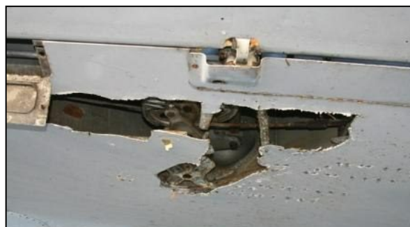
Figure 1 Corrosion Damage to wing bottom skin
