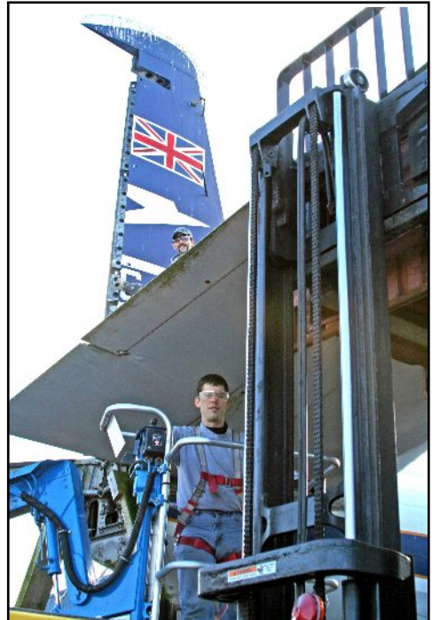
Bill Bush removing an elevator, supervised from above by Mike King
