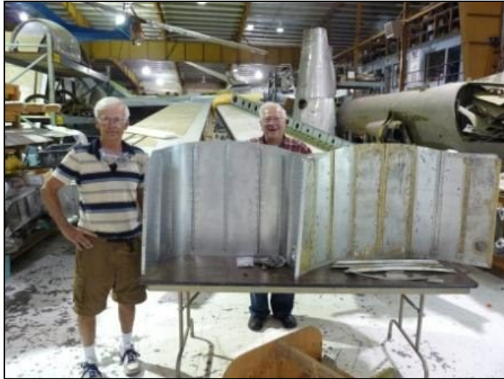
Figure 8 Aileron Control Bay – aft baggage compartment barrier --- before (right) and after (left).
