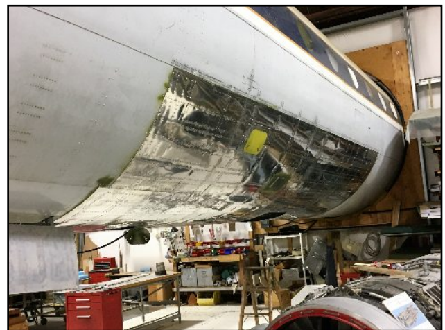
Re-skinned area of fuselage
