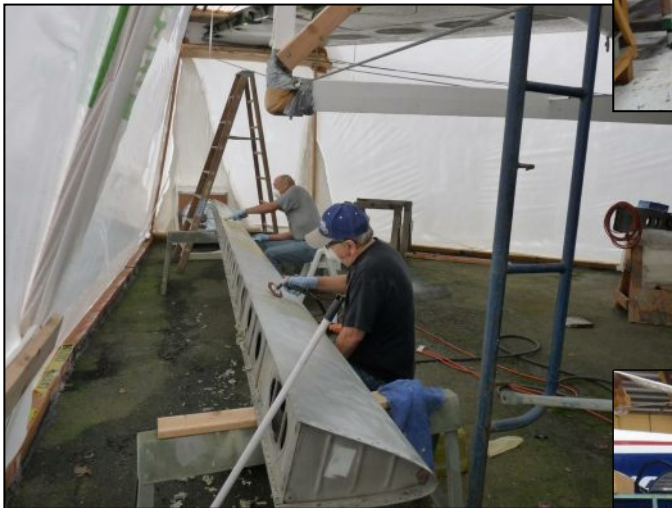
Part of vertical stabiliser under restoration.
