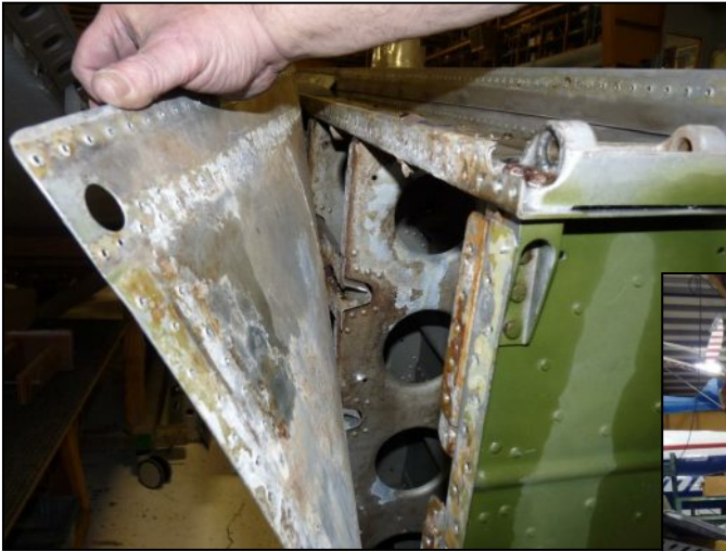
Horizontal stabiliser before restoration.
