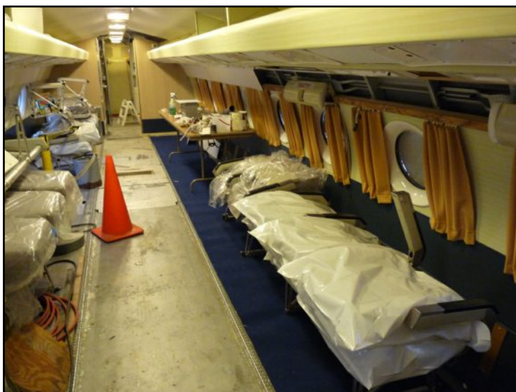
Aft cabin with trial carpet fitting, more window curtains in place. Note the grill in the center aisle floor.
