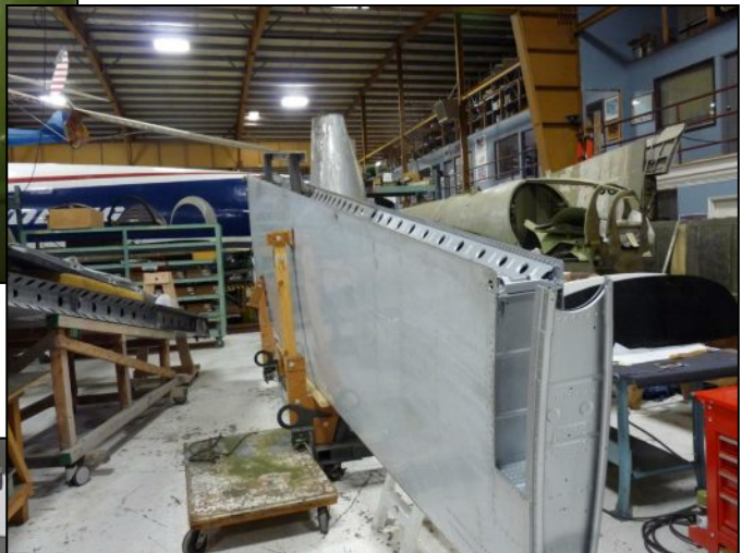
Horizontal stabiliser after restoration.
