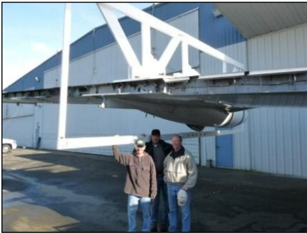
Figure 2 Pannier Tank Cable Support Beams
