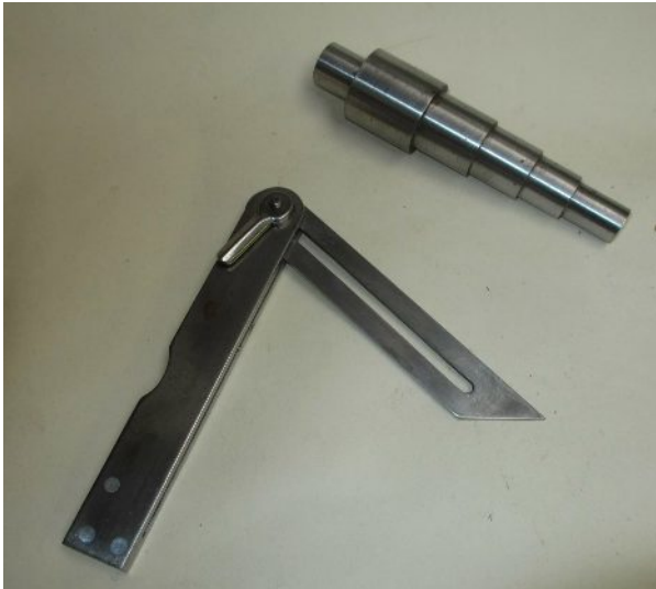
Turning with five diameters Steel angle gauge
