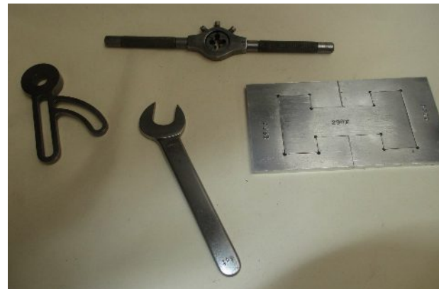
Two handled die holder plus die Spanner -11/16 A/F Fitting exercise - block within two blocks
