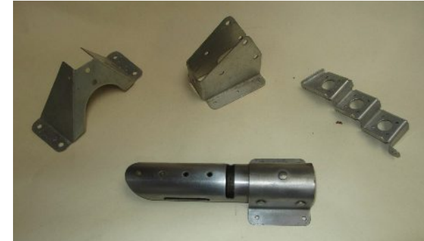
Pyramid flange Straight sided flange Three stepped angles plus centre holes and 1/16 rivet holes Tube and tube support
