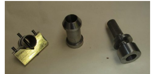
Tube in "v" plate with threaded studs Steel turning bored with tapered end Go -no go plug, end knurled
