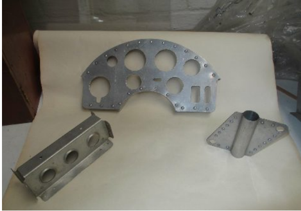
1/2 scale Moth instrument panel Flanged folding with lightening hole Tube and flange assy.
