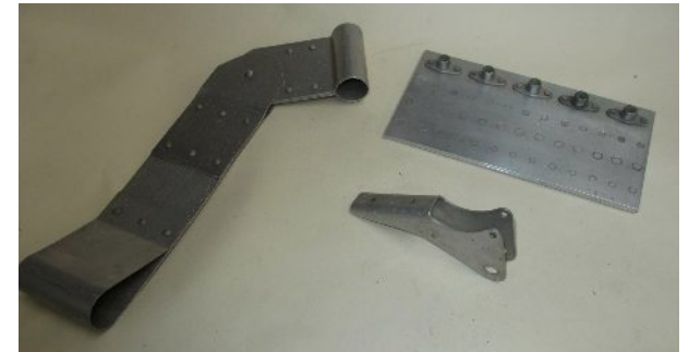
Sheet strip and hinged tubular end Rivet exercise - 39 rivets and 5 anchor nuts Small folded bracket
