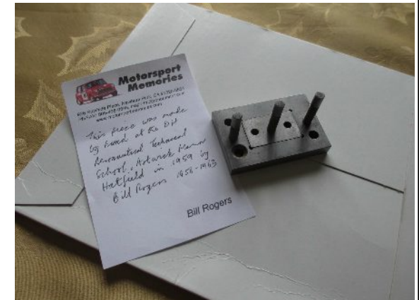
The first exercise given was usually to make a rectangular hole in a block into which another rectangle would fit perfectly. If this was done well the apprentice was allowed to drill and tap holes for threaded studs. This example was made by Bill Rogers in 1959.
