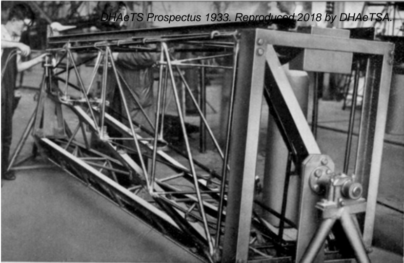
A steel fuselage in welding jig.
