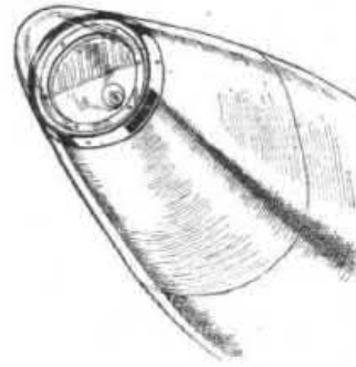
ROOM ENOUGH, BUT ONLY JUST: The diminutive cockpit of the "Comets." On the left, the landing light in the nose of the fuselage.
