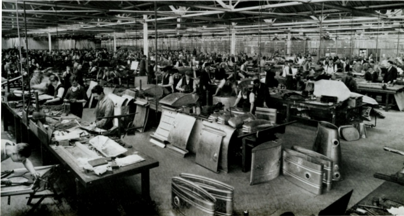
STUDENTS AT THE DE HAVILLAND AERONAUTICAL TECHNICAL SCHOOL pass through every department of the Company's factories. Above are views of (top) one of the erecting shops in the great modern works at Hatfield and (lower) the sheet metal shop with the machine shop in the background. The whole factory is laid out on the most modern scientific lines.
