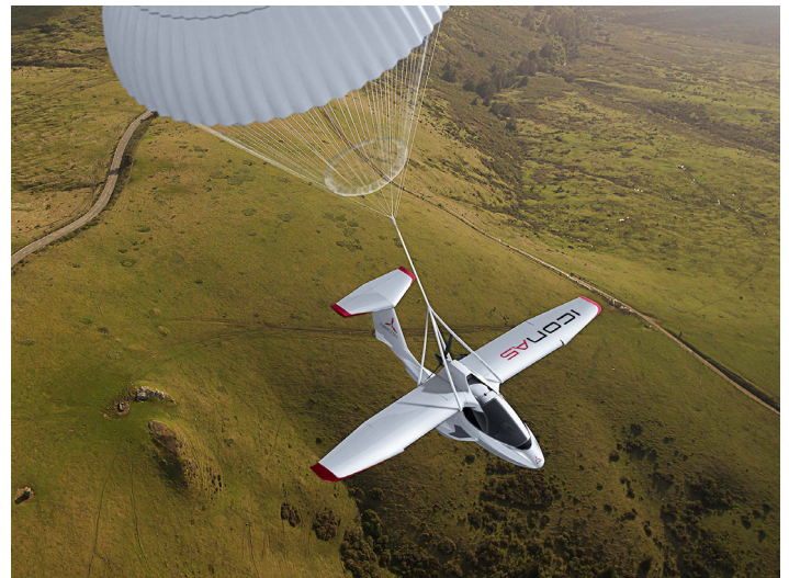
We don't normally wear parachutes, but some aircraft are fitted with ballistic parachutes for the whole airframe. Image: Ballistic Recovery Systems
